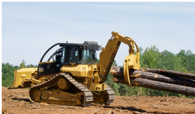
Figura 40: Track Skidder Caterpillar 527.
