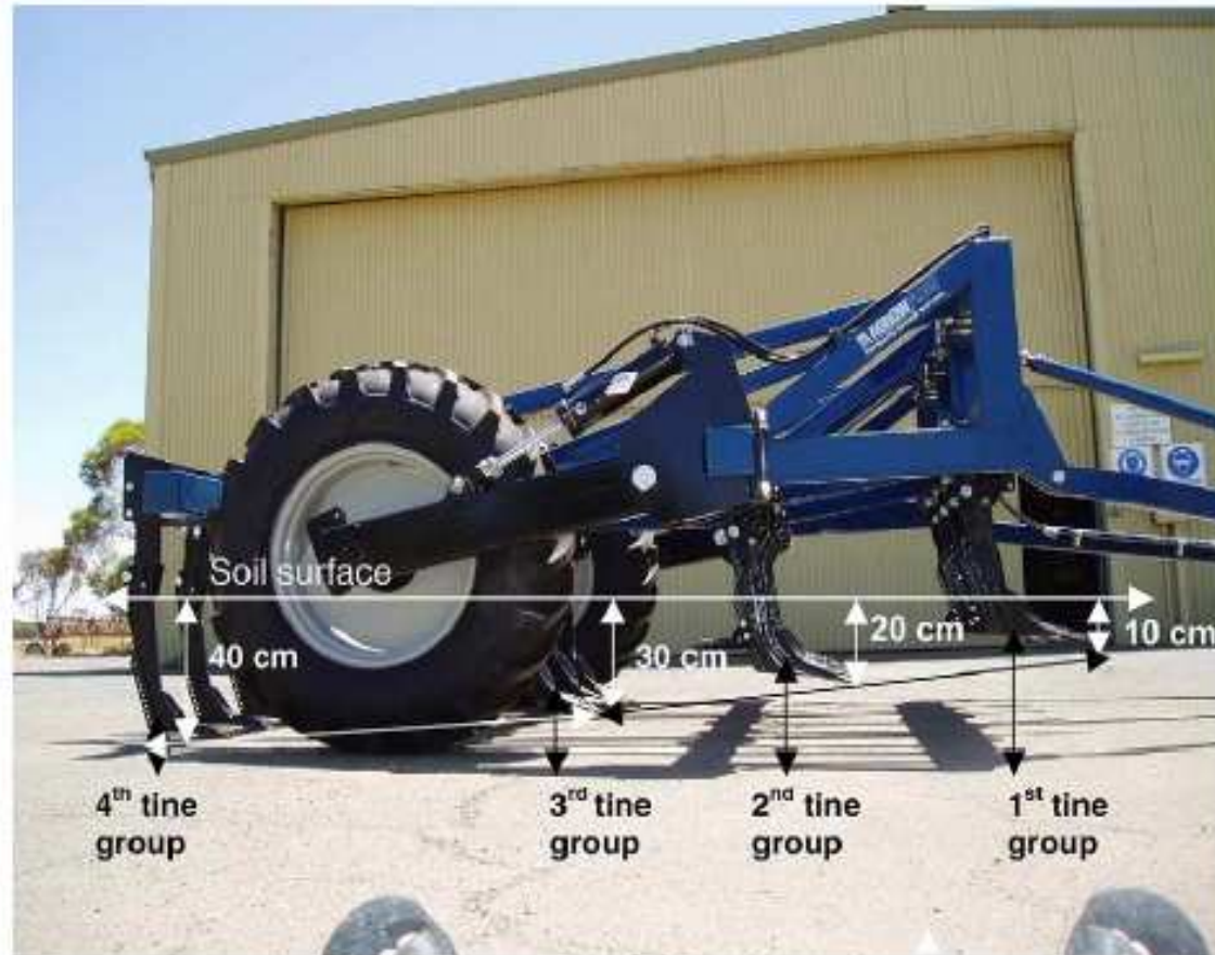
Fig. 3. A new generation ripper (Agrowplow ® ) applying the shallow leading tine concept where tines are aligned behind each other to rip consecutive soil depths. The first tine rips the first 10 cm of the soil, the second tine rips the next 10 cm, the third and the fourth tines each rip the next 10 cm. The total depth ripped by the four tines is 40 cm.
