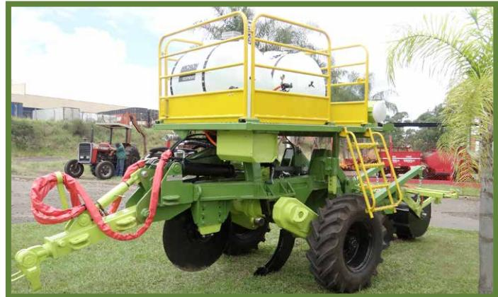
Aiming the development of technologies for the forestry line and aware of the roughness in this field, EcoAgricola developed the Forestry Subsoiler TERRAS F with reinforced structure. This equipment cleans the track where the work will be done, does the subsoiling up to 900mm deep, harrows the ground after subsoiling, marks the soil for the planting of seedlings and applies pre-emergent herbicide.
