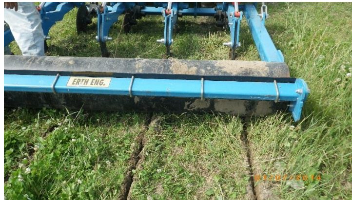
Efficacy of disks working at sufficient depth
