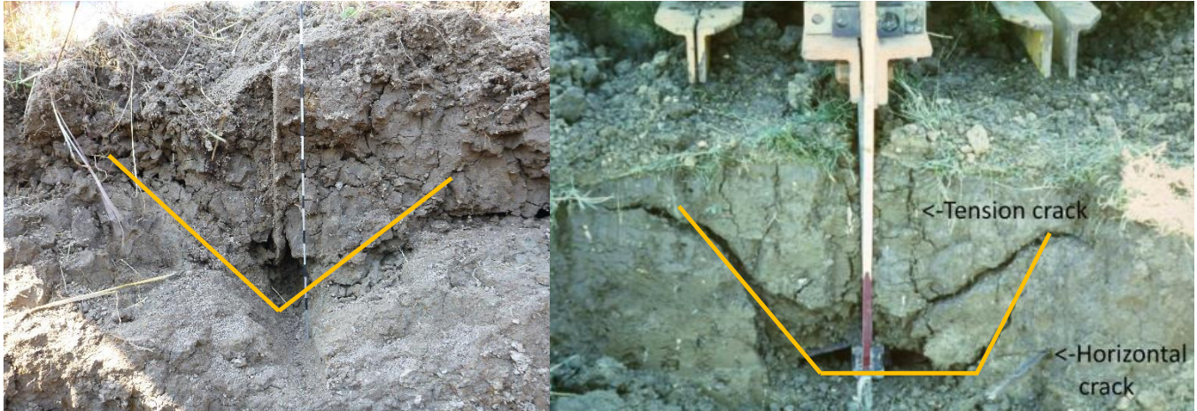
Narrow point: V shape of the loosened soil (a).
