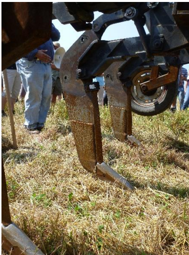
Figure 27. Straight cutting disks ahead of the tine leg which cut through the crop.
