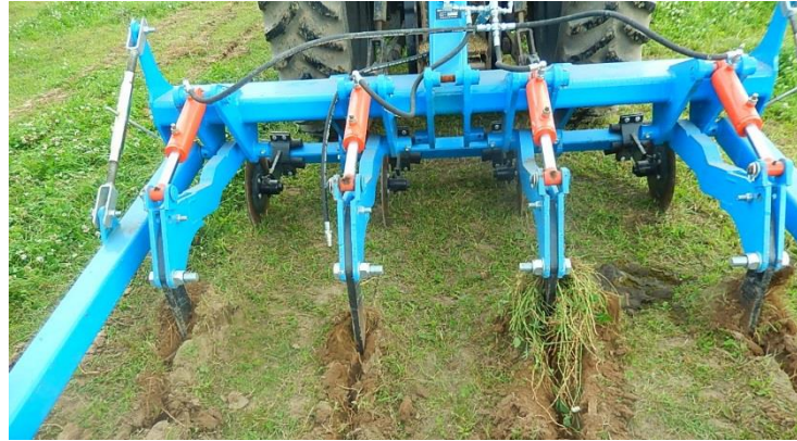
Figure 27. Straight cutting disks ahead of the tine leg which cut through the crop.
