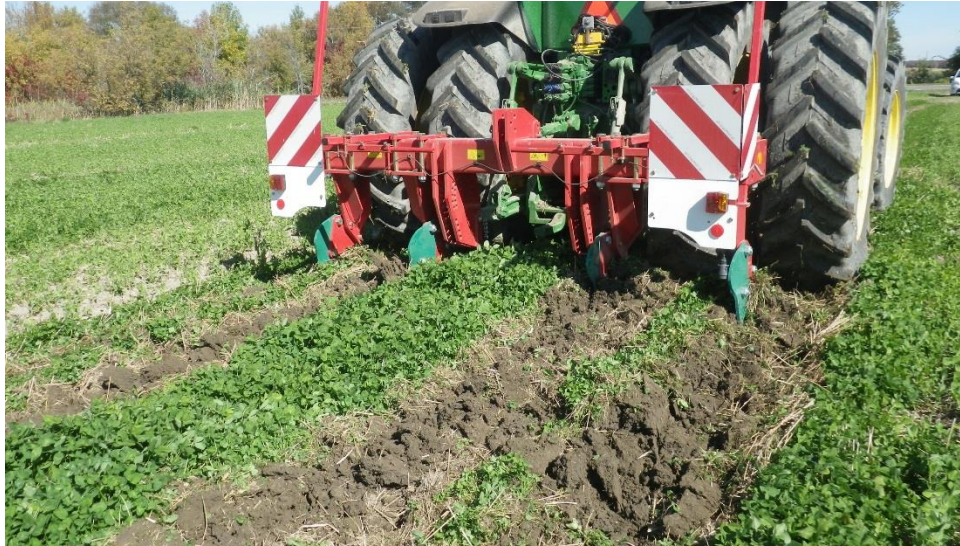
Figure 31. Excessive wheel slippage damaging the crop. In this photo the clods were raised above the surface by the combined effects of wheel slippage and the tines. The soil must be dry enough in order to perform such a procedure.
