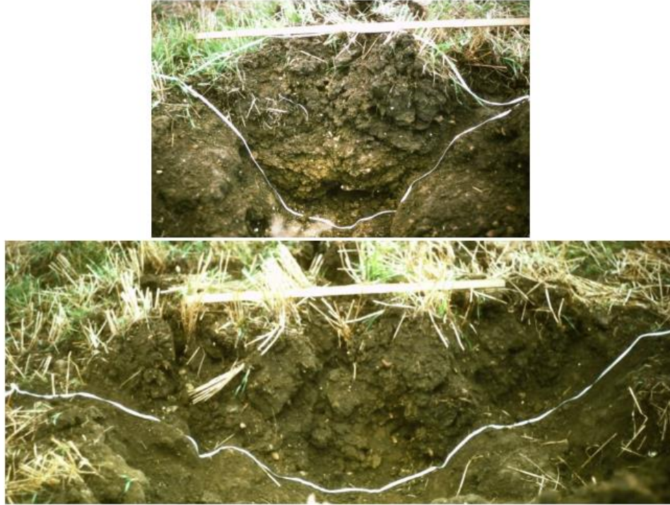
Figure 23. Soil disturbance from a winged tine only (top) and winged + shallow leading tines (bottom). Godwin and Spoor (2015) after Spoor and Godwin (1978). Reproduced with the kind permission of the authors and CABI.
