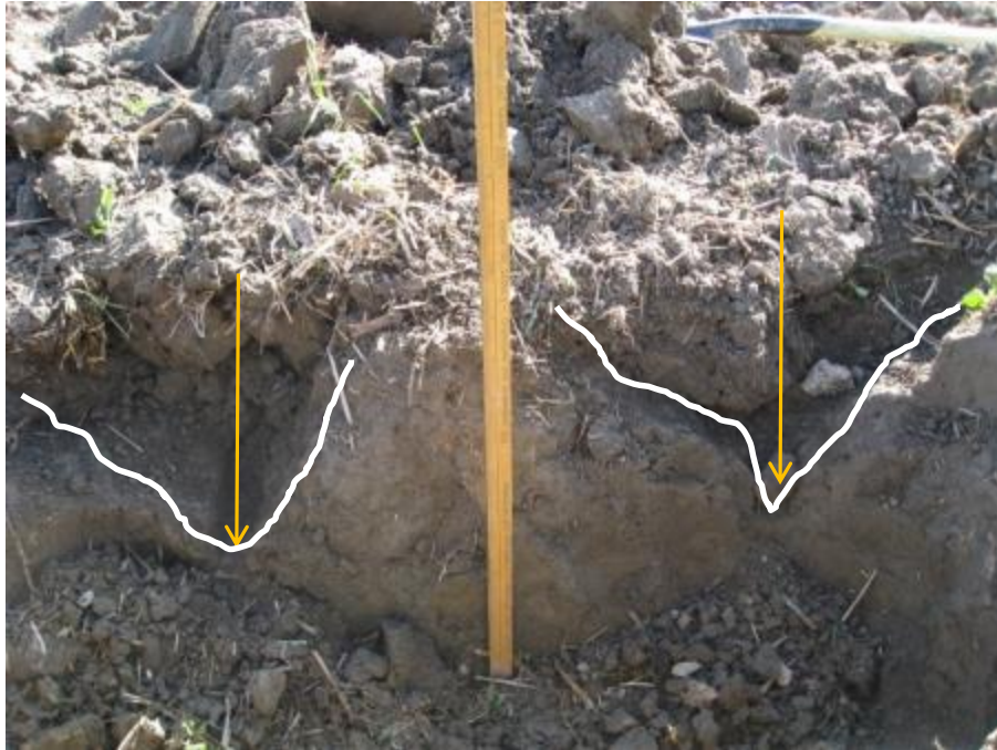
Figure 17. Partial soil loosening because of an insufficient working depth. In this case, the Vs do not overlap and only a small proportion of the soil has been loosened. The orange arrows indicate where the tines have passed.
