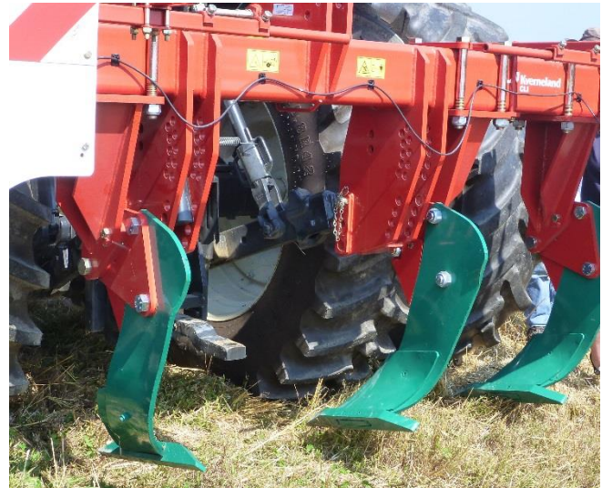
Straigh toolframe with one row of shanks.
