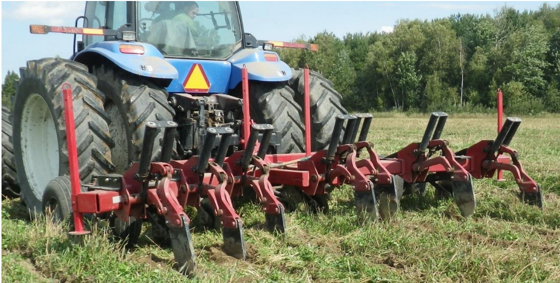
Figure 24. Tines that cannot penetrate a compacted sandy soil. The tine at the extreme right is the only one working at the desired depth while the one next to it cannot enter the soil properly.
