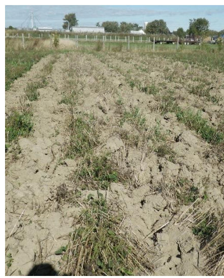
Figure 28. Effect of straight and curved tines on the surface disturbance of a clay soil
