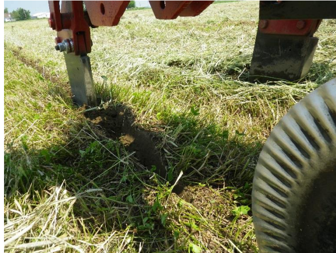
Disk placed ahead of the subsoiler's tine, avoiding damage to the hay crop as the subsoiler passes
