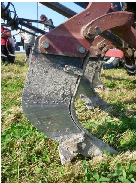
Leg with the upper part leaning forward (c).
