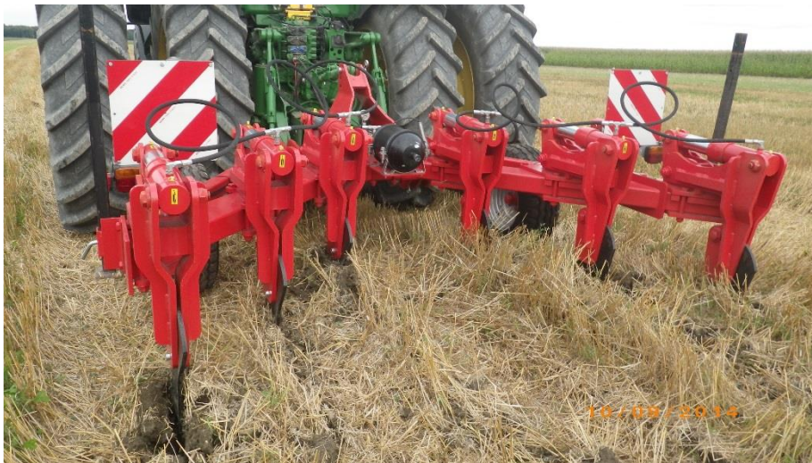
Figure 13. Slanted tine subsoiler with tine spacing of 50 cm (20") and working to a depth of 40 cm (16") in a clay soil. The small spacing between tines reduces the mass of soil that must be lifted by each individual tine, thus reducing the confining resistance.
