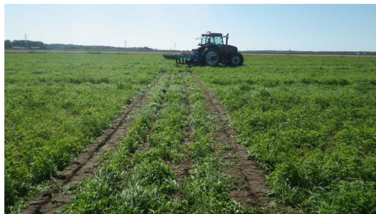
Figure 32. Panbuster subsoiler adapted for hay and pasture work. Straight cutting disks cut through the crop ahead of the tines. The tines have a low lift height and the packer roller crushes the clods.
