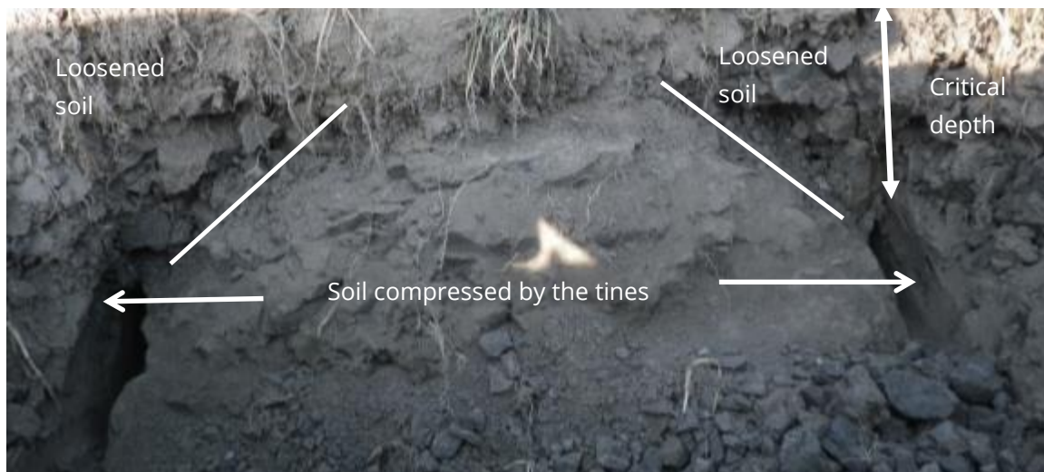
Figure 12. Brittle loosening above the critical depth and compression below it for a very compacted and moderately humid clay soil. The soil was fractured between 0 and 35 cm (14") depth and further compacted below that depth.
