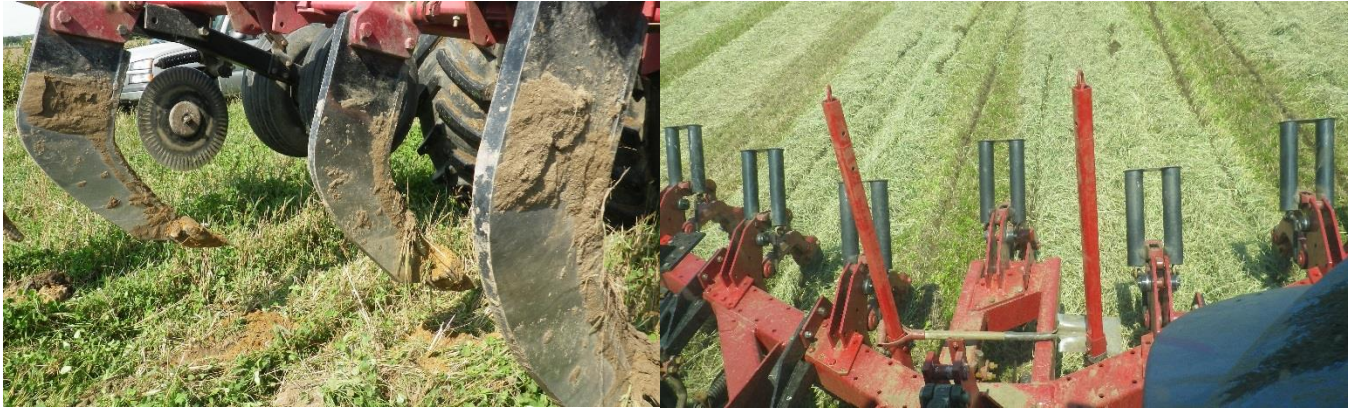
Figure 29. Use of curved tines in a sandy soil with disks cutting ahead of the tines in a clover and ryegrass hay field. Note: if the soil contains enough clay to form clods the crop will be damaged.
