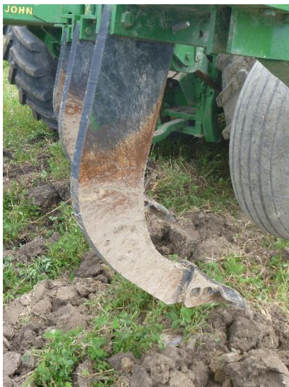
Figure 28. Effect of straight and curved tines on the surface disturbance of a clay soil
