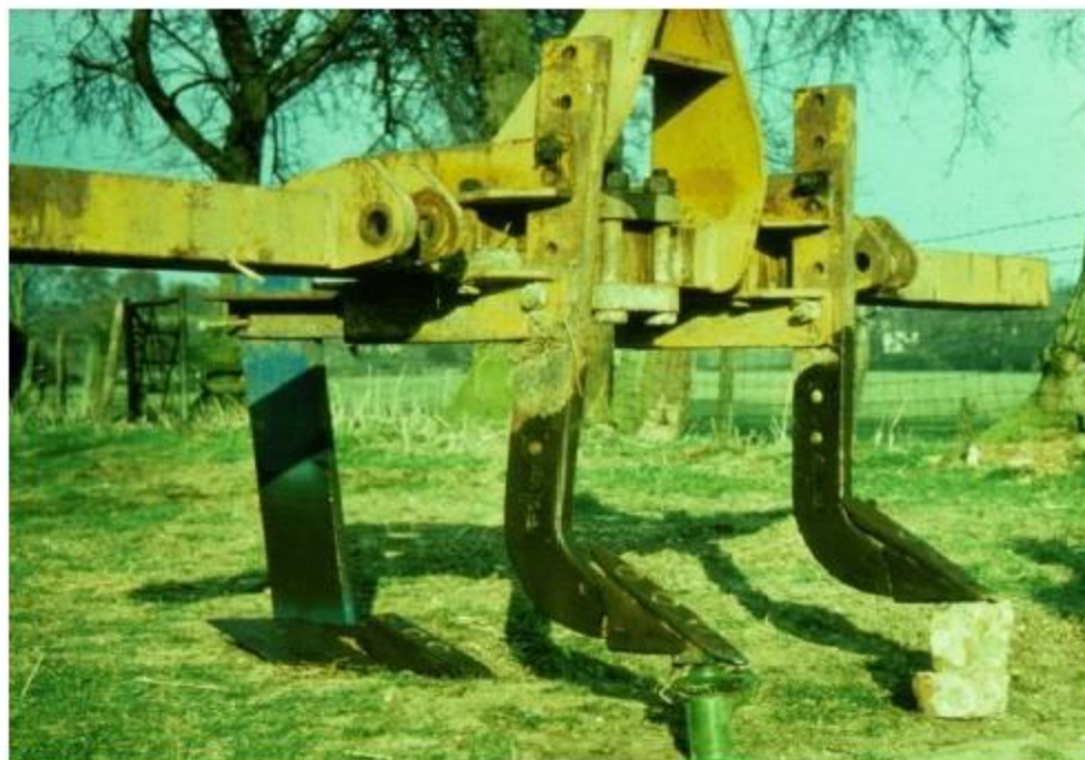
Figure 21. Subsoiler with shallow leading tines ahead of the deeper tines (photo by Dick Godwin).
