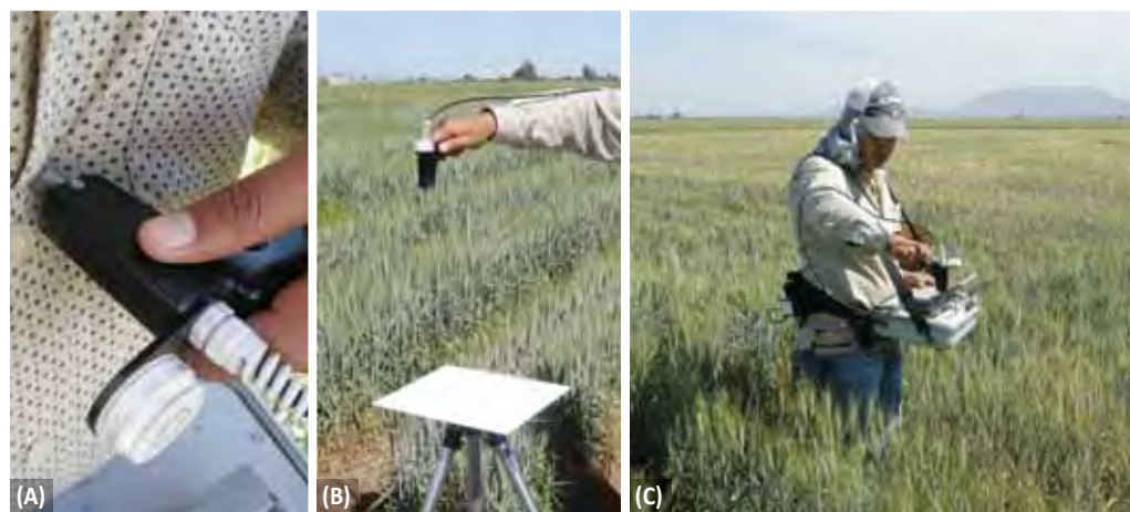
Figure 7.2. Taking readings with a field spectrometer: (A) dark reading; (B) white reading; and, (C) canopy reading.
