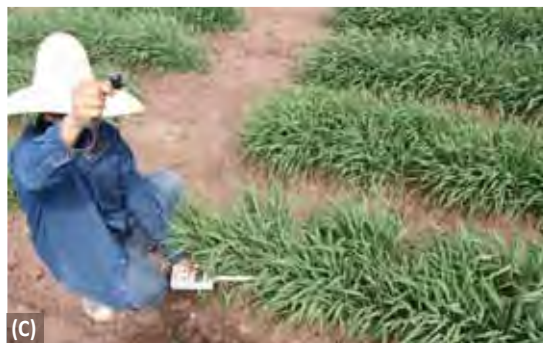
Figure 11.1. Taking light interception measurements with a hand-held ceptometer: (A) measurements below the spike; (B) the Decagon AccuPAR LP-80 ceptometer; and, (C) measurements at GS31, also showing the external sensor being held for simultaneous above-canopy measurements.
