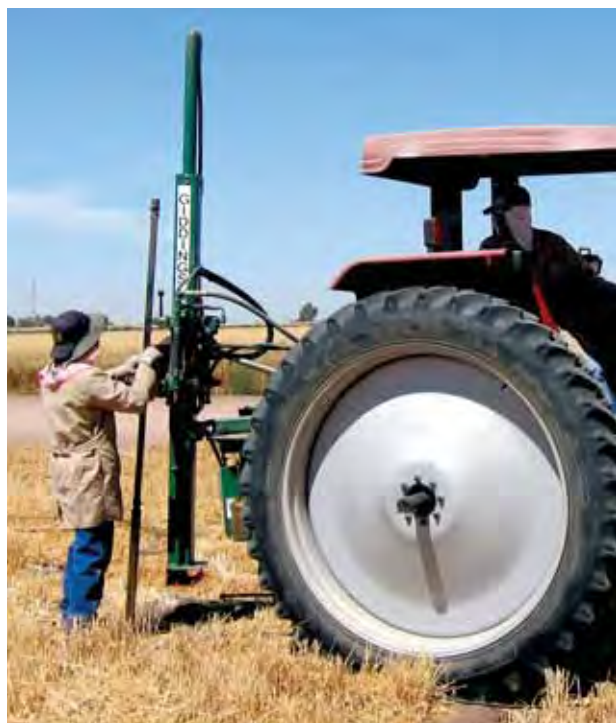
Figure 17.1. Soil coring using: (A) a tractor with 'Giddings' hydraulic soil corer; and, (B) a hand-held soil corer.
