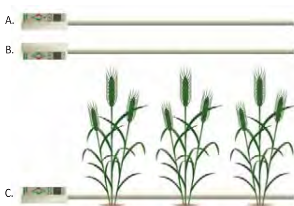
Figure 11.3. Taking measurements for calculation of light interception, of: (A) above-canopy PAR; (B) canopy reflectance (ceptometer turned upside down); and, (C) total canopy light interception.
