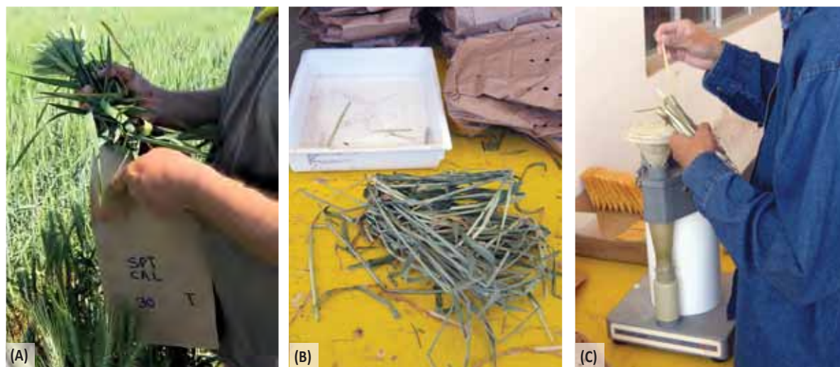
Figure 16.1. Sampling for WSC content: (A) taking 20 stems in-field; (B) removing by hand the leaf lamina and leaf sheaves from dry stems; and, (C) grinding dry stem sample using a cyclone mill.
