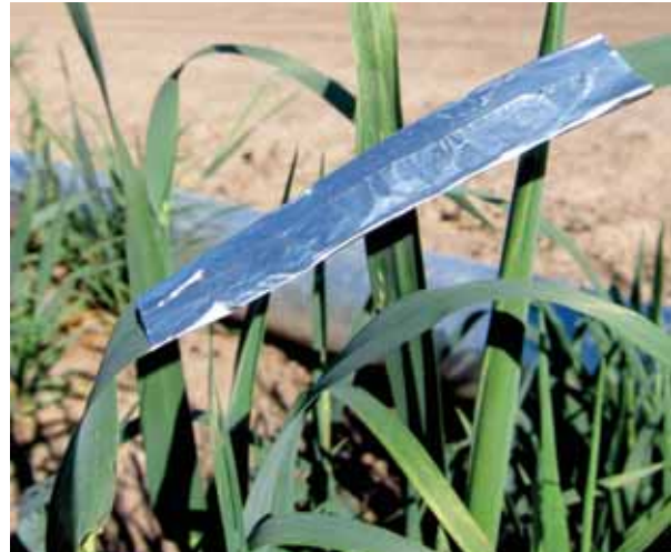
Figure 13.3. A self-made dark adaptation leaf clip using aluminum foil.
