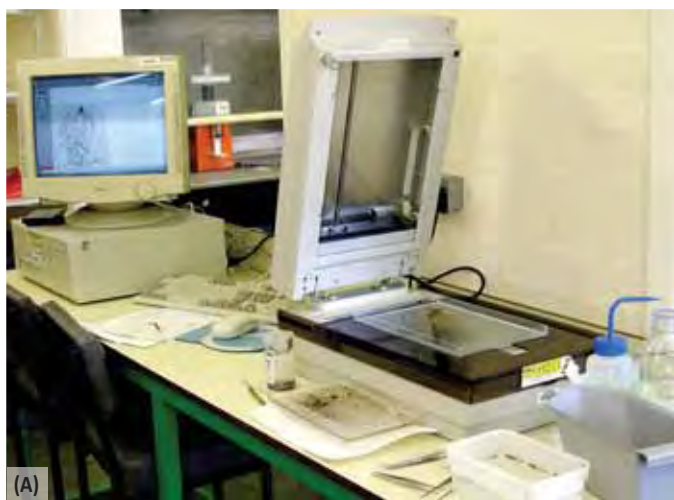
Figure 17.5. Root scanning: (A) root scanner (WinRHIZO STD 1600+, Regent Instruments Inc., Quebec, Canada); and, (B) scan of barley roots (Photographs: Pedro Carvalho, The University of Nottingham).
