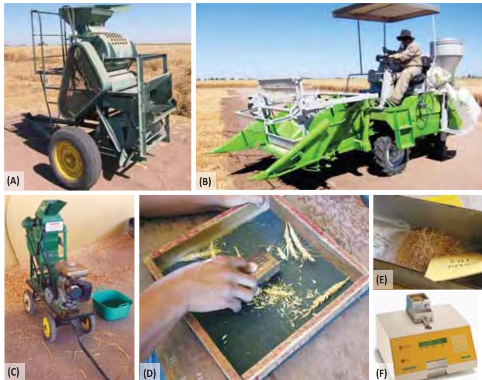
Figure 18.1. Harvesting for yield and yield components: (A) plot combine harvester; (B) large stationary thresher; (C) small stationary thresher; (D) hand-threshing a grab-sample; (E) a threshed grab-sample requiring final cleaning; and (F) a Contador seed counter (Pfeuffer GmbH, Kitzengen, Germany).
