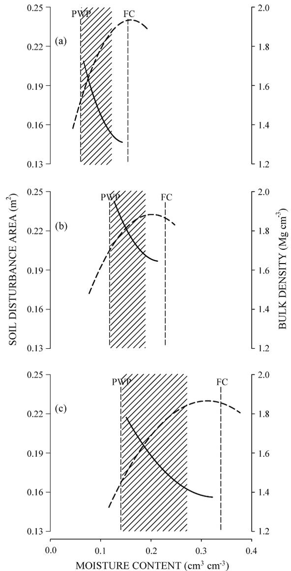
Fig. 8. Subsoiling water interval as a function of density (---), disturbance area (—) and water content in the soils: (a) loamy-textured Dark Red Dystrophic Latosol (LVd-1), (b) clayey-textured Dark Red Dystrophic Latosol (LVd-2), and (c) very clayey-textured Dark Red Dystrophic Latosol (LVd-3). PWP stands for permanent wilting point (−1.5 MPa); FC is the field capacity (−0.01 MPa). The hatched area represents the water interval at which subsoiling should be performed.
