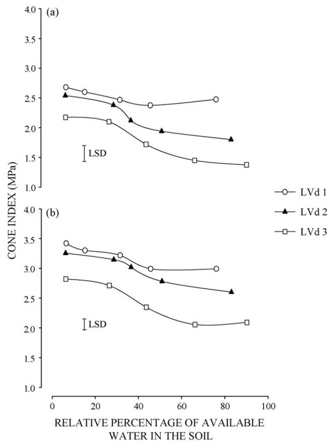
Fig. 4. Resistance to penetration variation as a function of relative percentage of available water in three Latosols: (a) 0–10 cm layer and (b) 10–30 cm layer. The error bars indicate the least significant difference at  $p = 0.05$ .
