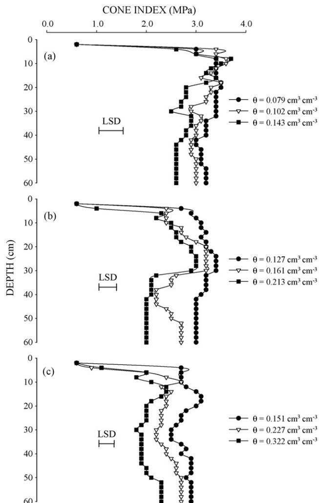
Fig. 3. Soil resistance to penetration, evaluated before subsoiling, under different water contents: (a) loamy-textured Dark Red Dystrophic Latosol (LVd-1), (b) clayey-textured Dark Red Dystrophic Latosol (LVd-2), and (c) very clayey-textured Dark Red Dystrophic Latosol (LVd-3). The horizontal error bars indicate the least significant difference (LSD) at  $p = 0.05$ .
