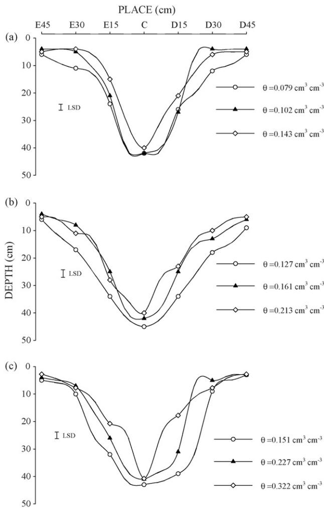
Fig. 5. Soil disturbance area as a function of water content: (a) loamy-textured Dark Red Dystrophic Latosol (LVd-1), (b) clayey-textured Dark Red Dystrophic Latosol (LVd-2), and (c) very clayey-textured Dark Red Dystrophic Latosol (LVd-3). On the X axis, point C is located on the central subsoiling row, and the others are located at a 15 cm distance to the left or to the right from one another. The error bars indicate the least significant difference (LSD) at  $p = 0.05$ .
