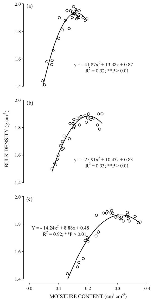
Fig. 6. Compaction curves obtained with standard Proctor test: (a) Loamy-textured Dark Red Dystrophic Latosol (LVd-1), (b) clayey-textured Dark Red Dystrophic Latosol (LVd-2), and (c) very clayey-textured Dark Red Dystrophic Latosol (LVd-3).
