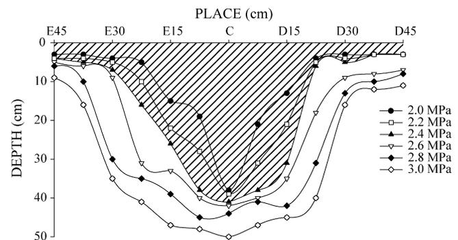
Fig. 2. Example illustrating soil resistance to penetration isolines, obtained with an impact penetrometer. On the X axis, point C is located on the central subsoiling row, and the others are located at a 15 cm distance to the left or to the right from one another. The highlighted area is delimited by the isoline that corresponds to the resistance to penetration before subsoiling (2.4 MPa); therefore, it designates the soil area displaced by subsoiling (SDA).
