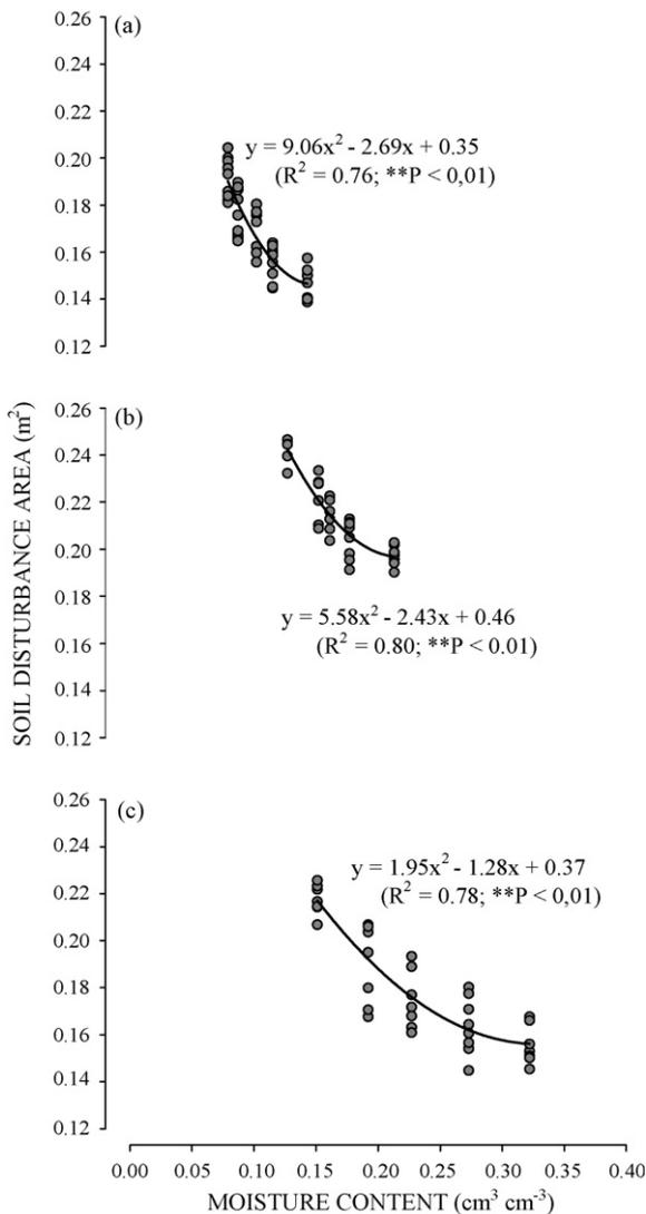
Fig. 7. Soil disturbance area as a function of water content: (a) loamy-textured Dark Red Dystrophic Latosol (LVd-1), (b) clayey-textured Dark Red Dystrophic Latosol (LVd-2), and (c) very clayey-textured Dark Red Dystrophic Latosol (LVd-3).
