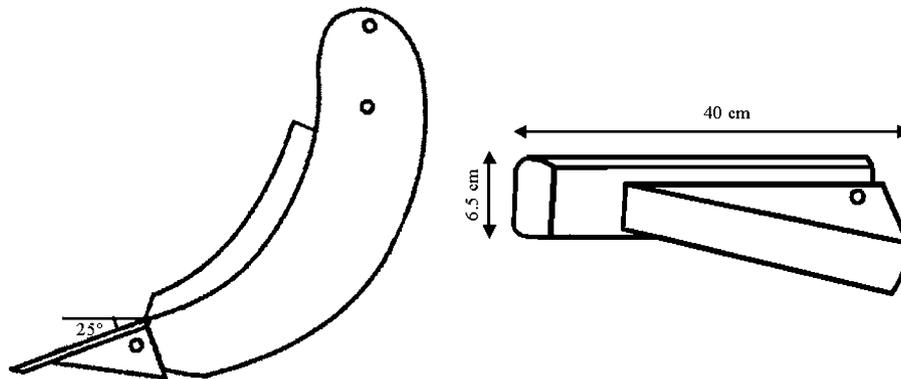
Fig. 1. Parabolic tine and dimensions of the subsoiler chisel without wings.
