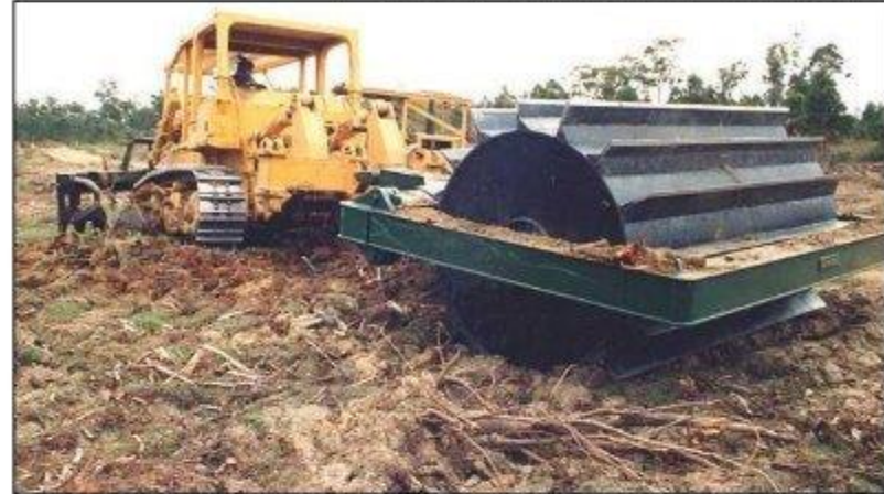
A Model 1120, 12 foot chopper equipped with a folding drawbar for transport requirements
