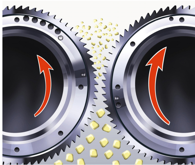
Figure 11.29 – Roll processor used to crush kernels and cobs in chopped corn silage (courtesy of Claas).
