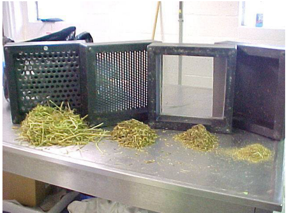
Figure 11.46. – Sieve set used to assess particle size distribution in forages and total mixed rations (Kononoff et al., 2003).
