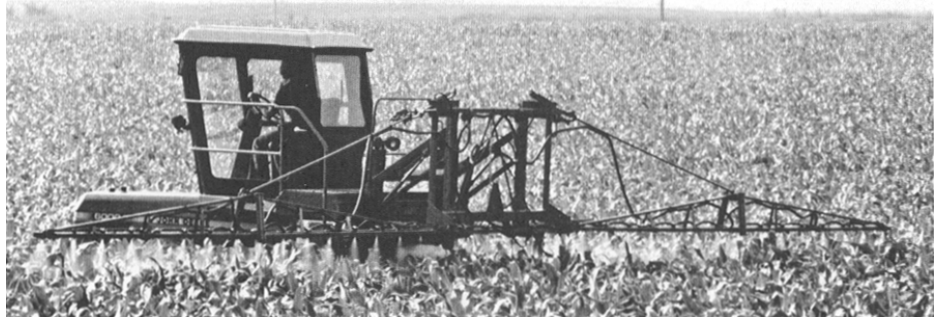
Figure 10.20 – A boom-type field sprayer (reproduced by permission of Deere and Co., © 1991. All rights reserved).
