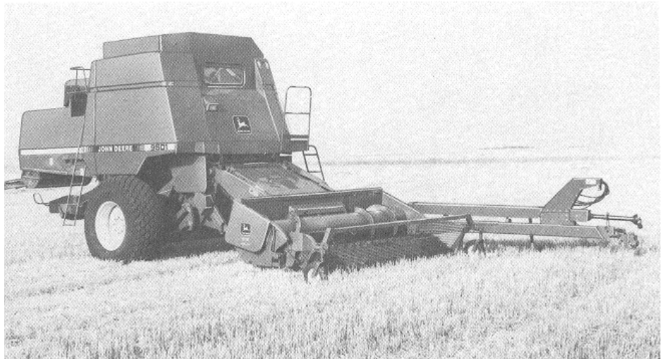
Figure 12.2 – A typical pull-type combine drawn by a tractor (reproduced by permission of Deere and Co. © 1991).
