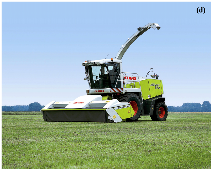
Figure 11.26 – Gathering units for forage harvesters: (a) pickup, (b) row-crop, (c) non-direction-sensitive, and (d) direct-cut (courtesy of Claas).
