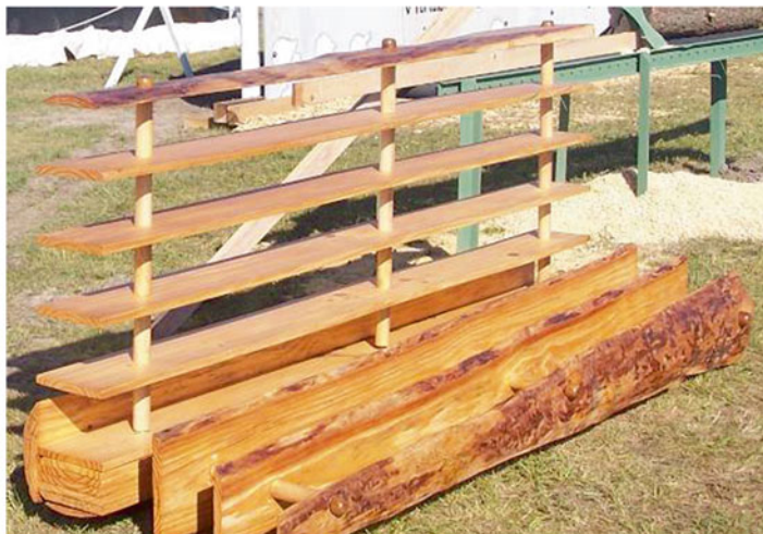
Fig. 2.11 Diagram and photograph showing the reconstruction of the cylinder that contains the defects (defect core) in the sawn log of a 17-year-old Pinus taeda (Fassola et al. 2002b)
