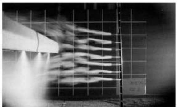
Fig. 4. Standard boom with F110/3-2/3-0 (coarse) nozzles spaced at 125 mm in air stream of 1.0 m/s with operating height of 500 mm
